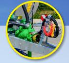
JUROP PN 106 pump protected in the V-shaped drawbar and air brakes in proportion to the load
