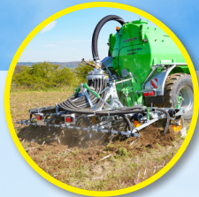
TERRAFLEX/2 XXL Working width: from 5.62 to 8.62 m
