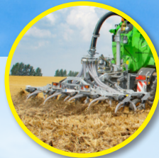
TERRAFLEX/3 Working width: from 4.4 to 6 m
