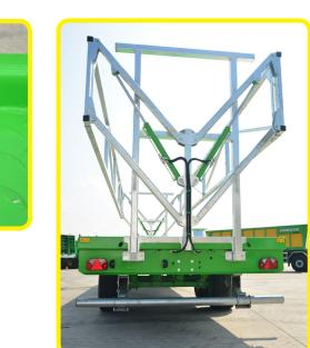
provides an ideal driving capacity, even in the hardest conditions. On the braking side, every axle is standard fitted with air brakes. 400x80 braking shoes are also standard available on all 6 wheels of the 20T versions; this bale trailer is therefore unquestionably an implement suited to high speed with a maximum load.
