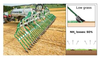
Next to these models are the so-called spreading booms "with skids". Based on a similar structure, they are additionally equipped with skids that exert a constant pressure on the ground by means of a system of spring leaves. By moving apart the vegetation, these skids ensure a precise distribution of the nutrients close to the plant base without dirtying the leaves or fodder. These implements are therefore ideal to fertilise
