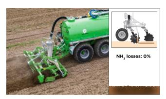
Next to these models with tines, the disc injectors offer a different action: equipped with 2 rows of curved and toothed discs, they work up to max. 10 cm deep. Their first row opens the ground, creating a groove in which the injection cones placed next to the discs apply the slurry. The second one, whose elements are positioned in the opposite direction as those of the first one, cover up and bury the slurry. Although these models
