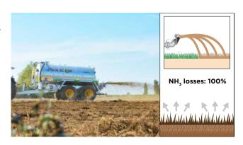
were released into the atmosphere and caused at the same time significant odour emissions. In some cases, it was therefore not uncommon to see a 100% loss of nitrogen!
