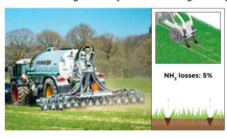
absorbed more quickly by the roots and ensures a higher and faster yield from the vegetation. This injection into the soil also prevents the release of more than 95% of odours and ammonia losses into the atmosphere, while reducing the risk of slurry leaching by unexpected rainfall. It should also be pointed out that, depending on the adjustment made on the machine, it will also be possible to use this type of injector for surface
